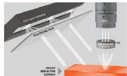
When paired with polarizing filters, polarizing film from Midwest Optical provides a complete solution for specular glare. The films can be cut to custom shapes and sizes to be mounted on almost any light source.
