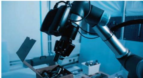
Two 3D camera achieves HD color 3D captures of typical bin-picking and piece-picking scenes in less than 0.3 seconds. The camera has a flexible working distance of 300 to 1500mm, and 57° horizontal by 35° vertical FOV. It measures 169x56x122mm, weighs 880g and has a dimensional trueness error less than 0.2%. By encompassing several vision inventions like pa-
