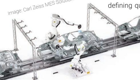
The system provides high-precision digital quality information through point cloud-based feature detection in real time. The system contains a fixed floor markers with integrated
