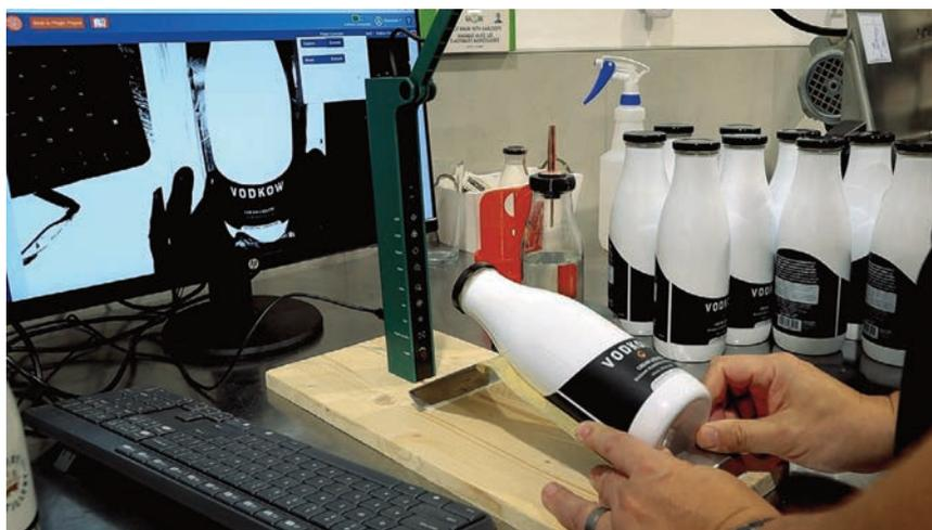
Image 2 | A fully integrated visual inspection system includes a camera, display, edge processing, and pre-packaged common inspection skills.
