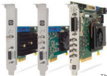
The Coaxlink frame grabber family of Euresys is growing with the addition of one- and two-connection CoaXPress CXP-12 boards.
