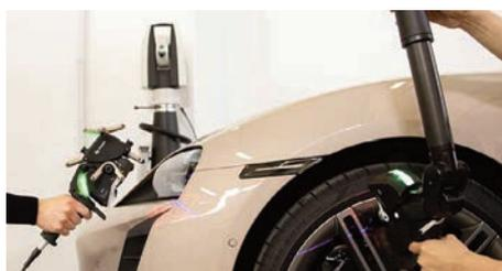
Scanner AS1 with an automation-capable data collection speed of 1.2 million points per second and interoperability between portable arm and laser tracker systems. The same scanner can be moved back and forth as needed between an arm used for interior quality control and a tracker setup performing flush and gap inspection. The scanner has a modular blue
