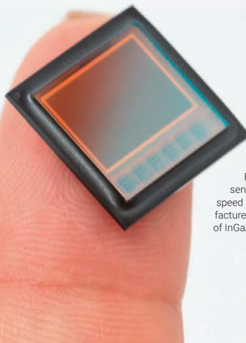
**Image 1 |** The CMOS-based SWIR sensor Raven has a resolution of 1,284X960 Pixel, a sensor spectrum of 0.4-1.6 $\mu$ m and a maximum speed of 120fps (full frame). The sensors are manufactured at a cost one thousand times lower than that of InGaAs-based SWIR sensors.
