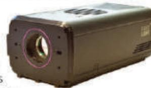
The 640x512 InGaAs SWIR camera C-Red 2 now offers a read out speed performance of 600 images per second full frame while keeping its performance of 30 electrons readout noise. Either in USB3 or Camera Link interface and easy as plug&play, users can enjoy high speed SWIR imaging for scientific and industrial applications.
