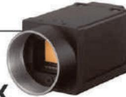
The XCG-CP510 camera is based on Sony's IMX250MZR global shutter CMOS sensor, which uses monochrome quad polarised filters to capture polarised light in four planes. To extract the best possible image from the CMOS, the design of the small camera module (29x29x42mm) has been optimised and outputs 5.1MP polarised B/W images at 23fps, transmitted over a GigE interface. The XCG-CP510 outputs 23 2,448x2,048-pixel frames per second. Additionally, an exclusive polarised-camera SDK is available.
