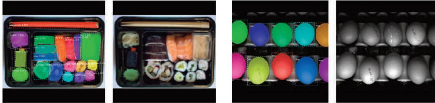
Images 1 + 2 | Modern deep learning networks can be trained with typically 20 to 50 training images within five to ten minutes on a modern GPU platform, e.g. object classification of sushi meals.
