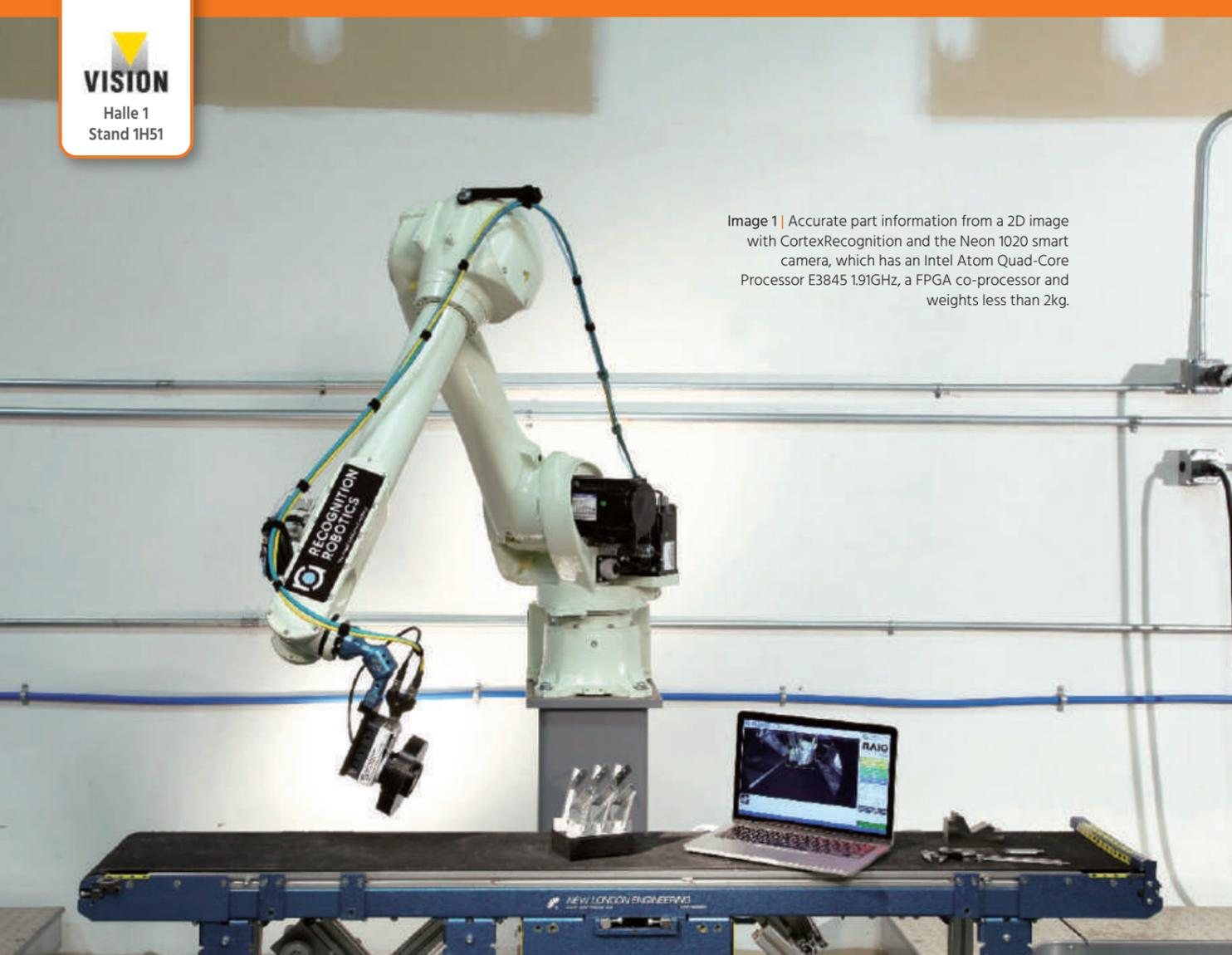
Image 1 | Accurate part information from a 2D image with CortexRecognition and the Neon 1020 smart camera, which has an Intel Atom Quad-Core Processor E3845 1.91GHz, a FPGA co-processor and weights less than 2kg.
