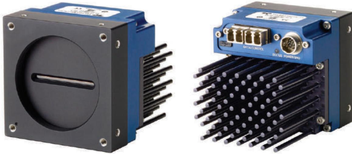
The color and multispectral camera Linea ML delivers images at a maximum line rate of 300kHz aggregate line rate in 8k/16k resolutions using the next generation CLHS fiber-optic interface.
