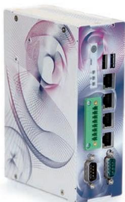
The BoxFlex XS is a compact version of the BoxFlex industrial PC series of Pyramid. Thanks to the optional DIN rail mounting and four possible 1GB/s network interfaces, the ipc is suitable as an edge device. Dimensions are 155x110x50mm, a 3,5 inch form factor and a 10W CPU power dissipation (TDP).
