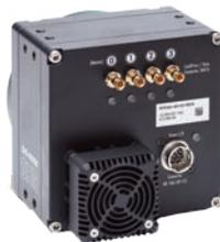
ons. For easy integration an I/O framework with multiple inputs and four power-out outputs is provided, supporting precise triggering as well as sequencers and logical operators. The outputs with the built-in strobe controller can directly drive LED lighting.
