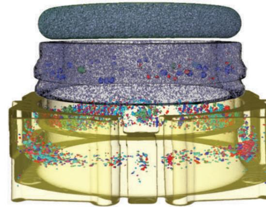
Image 2 | Defect analysis on a multi-material automotive connector using Avizo Software. Data courtesy of RX Solutions.
