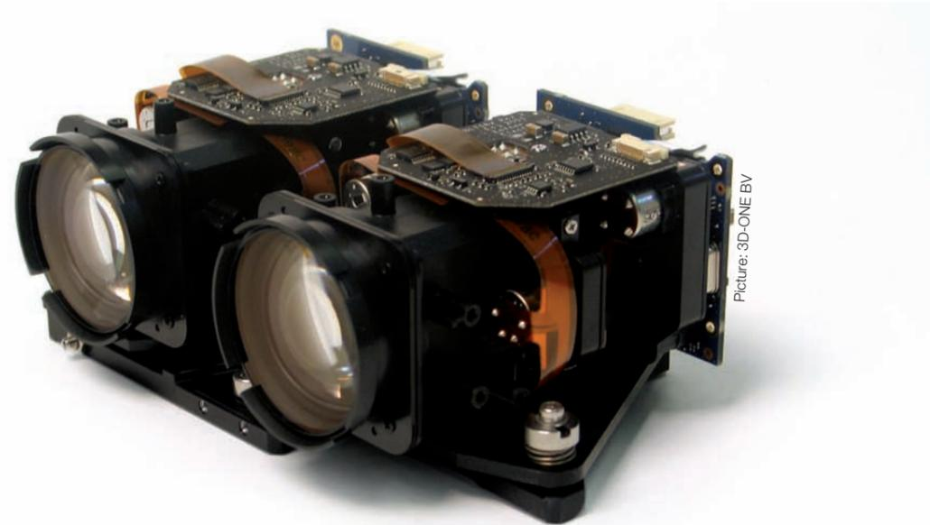
The embedded platform Stereoview is able to capture and display full HDTV images in real time and combines 3D stereoscopic imaging with optical zoom and auto-focus functionality
