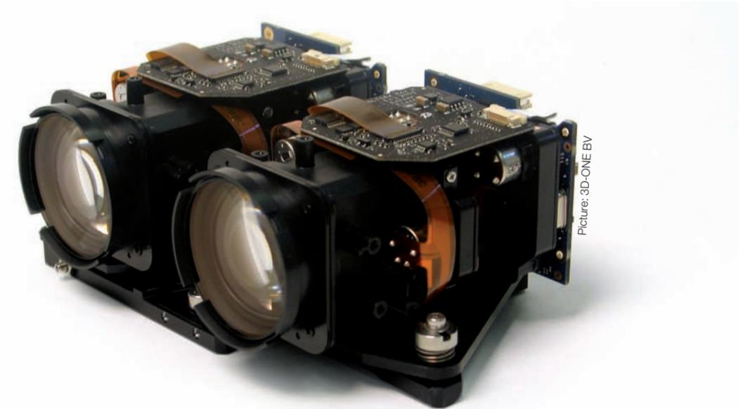
The embedded platform Stereoview is able to capture and display full HDTV images in real time and combines 3D stereoscopic imaging with optical zoom and auto-focus functionality
