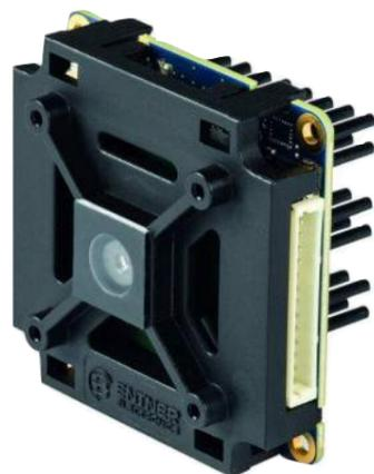
The UC-200 is a compact camera that allows for easy integration into embedded vision systems. It utilizes a Sony 13MP Exmor (rolling shutter) sensor operating at 30fps and an integrated F2.2 lens. The proprietary camera read-out electronics are optimized for a low latency. The camera supports 1080p/60 HDMI or LVDS
